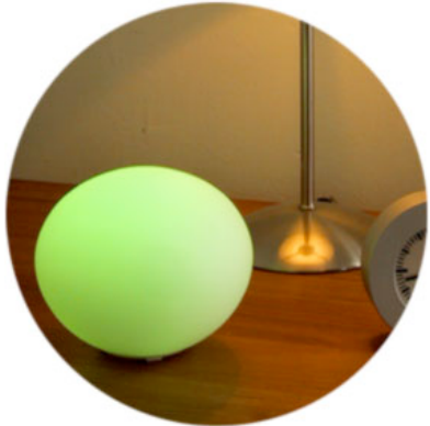
Figure 1. The Ambient Orb from Ambient Devices consists of a small frosted glass sphere that can shift between thousands of colors, and is controlled wirelessly by a cellular pager network.
